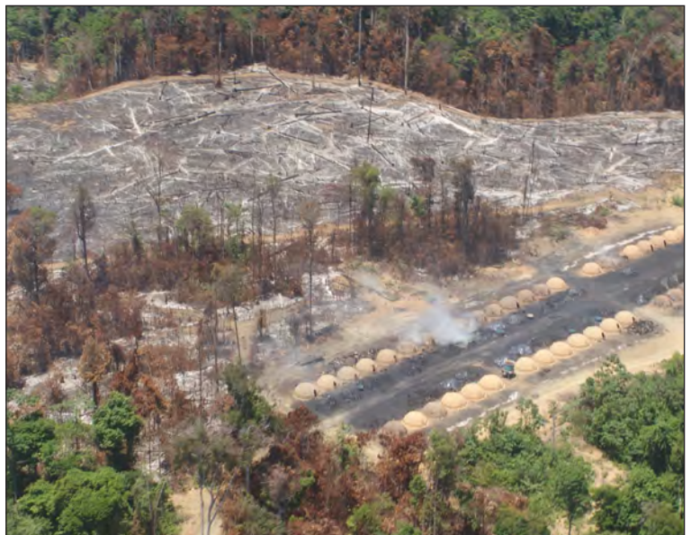
Rows of beehive ovens used for a charcoal operation in Pará state, Brazil. Photo credit: Eric Stoner.
